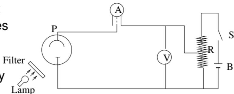
*Reverse-biased arrangement for studying photo-electric effect.*
