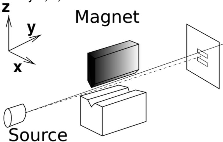
*A schematic diagram of the Stern-Gerlach experiment.*
